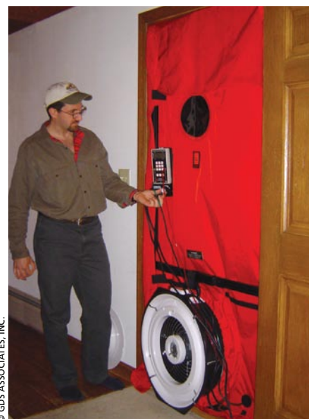
A residential energy efficiency specialist performs an air infiltration (or blower-door) test on a New Hampshire home. The test measures the tightness (or leakiness) of a building; results may indicate the need for sealing of cracks and voids (around doors or windows, for example) where heat is being lost.
