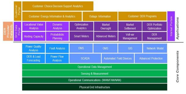
Green - Core Cyber-Physical Layer (including poles and wires) Blue - Core Planning & Operational Systems Purple - Applications for Planning, Grid & Market Operations Gold - Applications for Customer Engagement with Grid Technologies Orange - DER Provider Application
