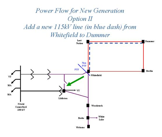
III. To accommodate 400 – 500 MW of additional generation resources connecting between Littleton and Dummer, a new higher capacity 230-kV transmission line could be constructed
